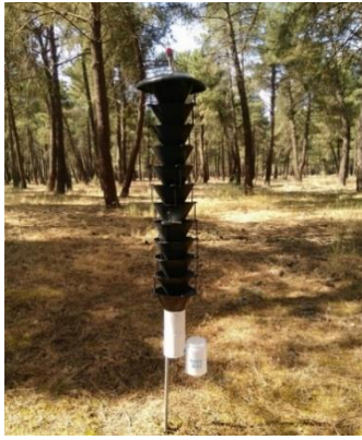
Multi-funnel trap baited with pheromone used to trap M. galloprovincialis | Photo: UVa
